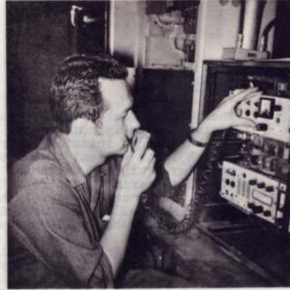
Milan, VE2AVP, operating the 450 Mhz. equipment. The control system is visible beside the 450 gear.
